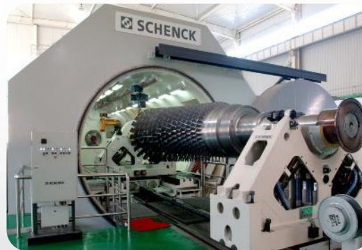
32t high-speed dynamic balancing machine
